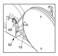
Drive Belt, you must remove both side shields. Refer to the instructions at the left and remove the side shields.
